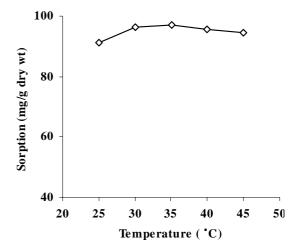
**Fig.2.** Biosorption of strontium from solution by *Bacillus* sp. GT-83 at various temperatures.
