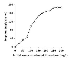
Fig.3. Effect of various initial concentrations of strontium on the biosorption capacity of *Bacillus* sp. GT-83.
