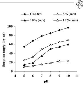
**Fig.1.** Biosorption of the strontium from solution by *Bacillus* sp. GT-83 at various pH and ionic strength values as MgCl<sub>2</sub>.
